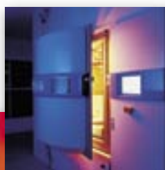
In ultra-modern vacuum coating facilities, a reflex-reducing layer is applied
