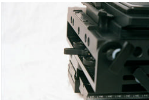
Note that the swing lever sticks almost directly out when locked down.
