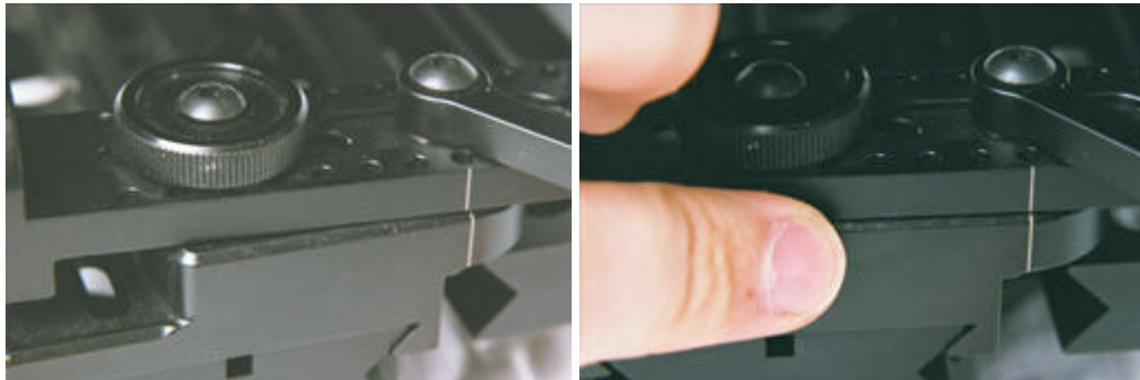
Left: Exaggerated example of unintentional swing. Right: Use your index finger to check for swing from the rear, or visually check for swing.
