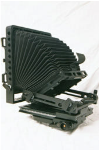
DLC with rear standard up, and front standard partially unfolded
